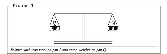
Iron wool is placed on pan P and weights are added to pan Q to balance the scales. The iron wool is removed and heated in the air. It forms a black substance which must be carefully collected and returned to pan P. Now the students can see, that the "black iron wool" weighs more than before. We have to explain that iron reacts with oxygen of the air to a new black substance called iron oxide. The amount of oxygen causes the higher mass.
